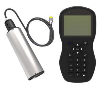
The BOQU portable turbidity meter consists of a host and a turbidity sensor. The turbidity sensor is based on a combined infrared absorption scatter ray method, and the ISO 7027 method can be used to continuously and accurately determine the liquid turbidity. The turbidity value was determined according to ISO 7027 infrared double scattering light technology without chromatic influence.
