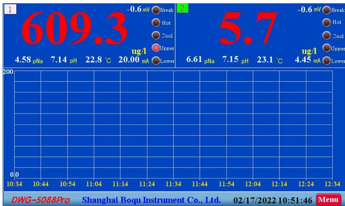
The table in the middle of the interface shows the real-time curve of measurement results. The real-time curve of the first channel is red, and the real-time curve of the second channel is green.
