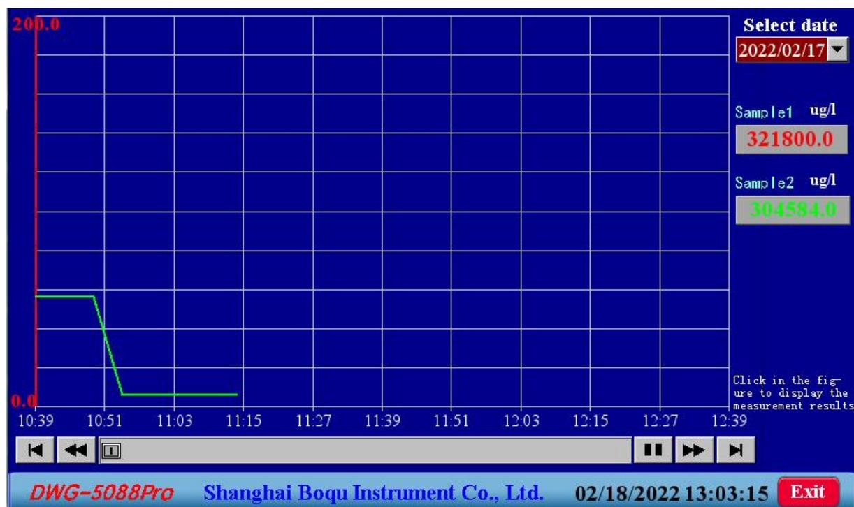
You can drag the scroll bar below the curve to view the historical curve of the day back and forth. Click any position on the curve, and the measured value of corresponding time will be displayed in the right data box.
