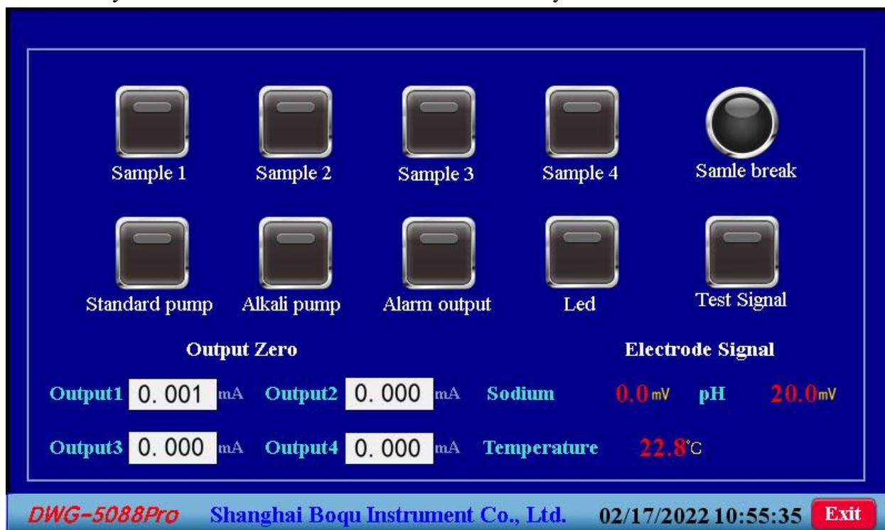
There are 8 buttons on this interface, corresponding to 4 sampling solenoid valves, 2 pumps, 1 alarm switch and 1 LED indicator. Click the button to open or close the corresponding parts, which is used to detect whether the action of each part is normal.
